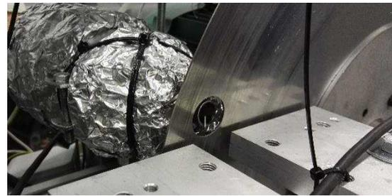
Figure 50: Thermocouple characterization apparatus, a (left) air heater, b (right) air jet
