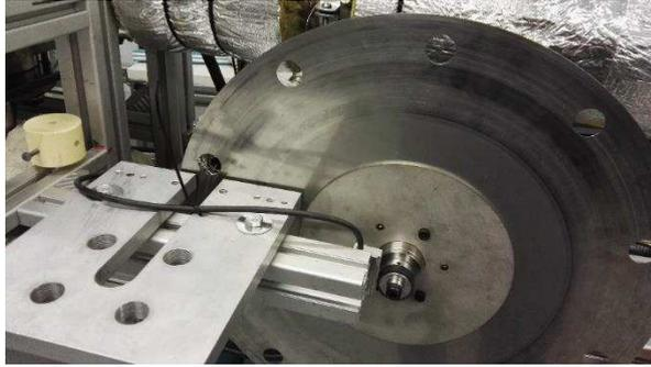
Figure 49: Thermocouple characterization apparatus – Rotating wheel
