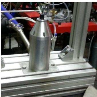
Figure 41: Air jet + Hot-wire probe
