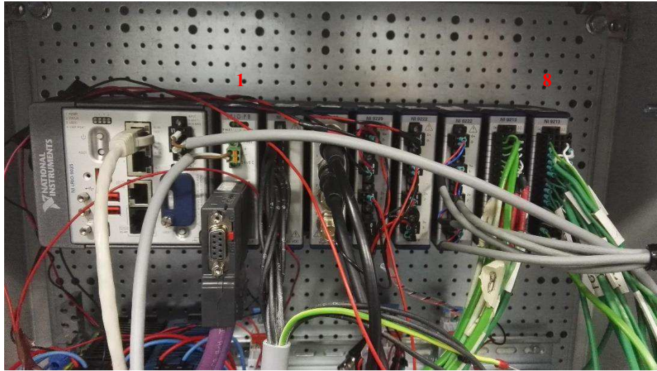
Figure 35: NI-9035 cRIO – final configuration
