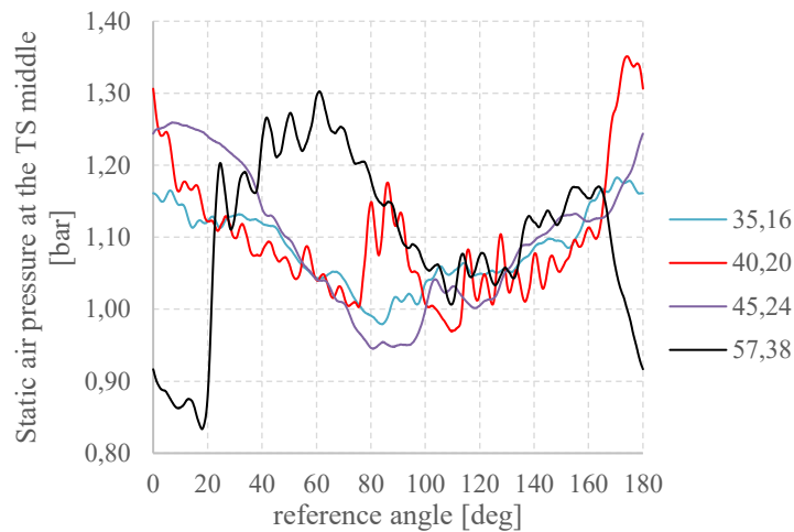
Figure 87: Static air pressures at the middle of the test-section for different pulsation frequencies
