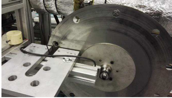
Figure 49: Thermocouple characterization apparatus – Rotating wheel
