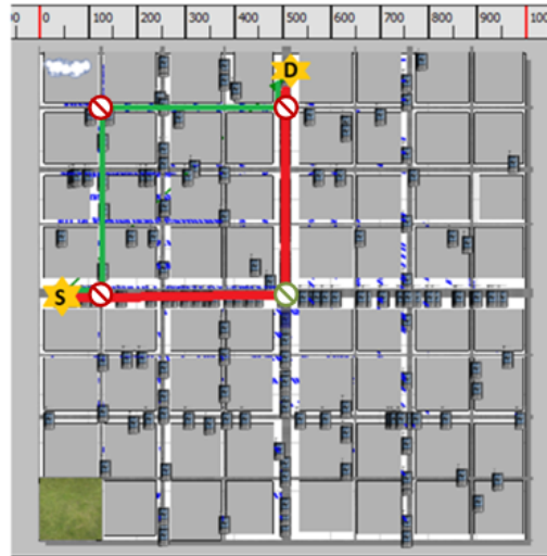
FIGURE 6.4: Direct (green) versus diverted (red) path between source and destination, d_F = 3 , n = 200
