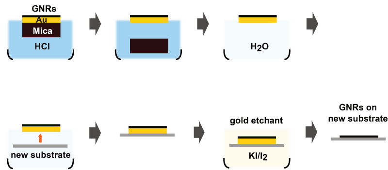
Figure 3.3: Transfer process of 9-AGNRs from the growth Au/Mica substrates onto the target glass substrates.
