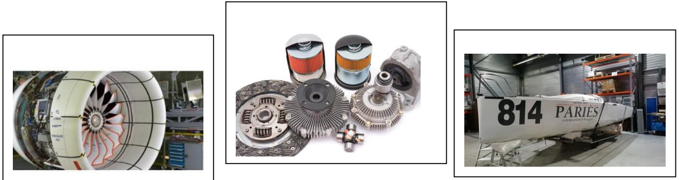
Figure 1.1. Applications of composite materials. Left: CMC on a jet turbine 1 . Center: MMC on automobile spares 2 . Right: OMC on a sailing ship 3
