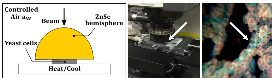
Figure 7-1 : Schematic representation of the ZnSe hemisphere, images of the stage used and the double-stained yeast L. thermotolerans cells. The cells were fixed to the surface of the ZnSe hemisphere and carefully placed at the base of the stage. The synchrotron beam was calibrated in the center of the hemisphere. The air relative humidity and temperature were controlled and monitored during dehydration kinetics and acquisition of spectra. Only green-live cells were selected before dehydration .
