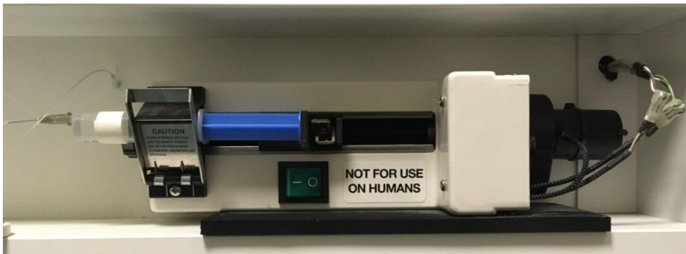
Figure 21. External pump for i.v. saline or COC infusions.
