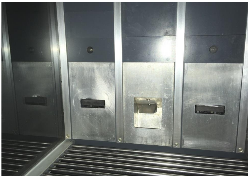
Figure 22. Operant conditioning cages for food pellets with two levers in each side of a food magazine.
