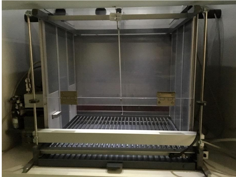
Figure 20. Operant conditioning chamber fitted in wood attenuation boxes.
