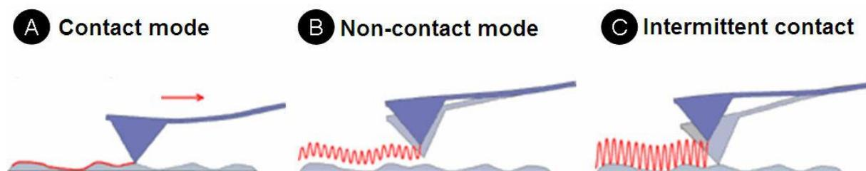
**Figure 7.** Contact (panel A), non-contact (panel B) and intermittent contact (panel C) modes of operation. Figure adapted from Ref.<sup>27</sup>
