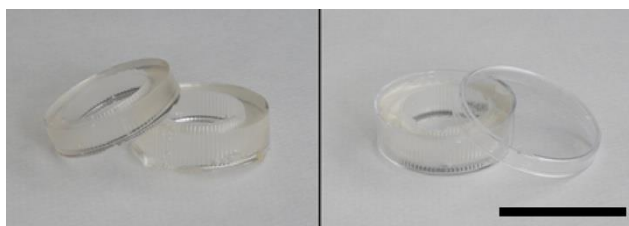
Figure 3.10. Images of PDMS holder (left) used for holding the coverslip in 3 ml Petri dishes (right). Scale bar 3 cm.
