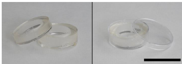
Figure 3.10. Images of PDMS holder (left) used for holding the coverslip in 3 ml Petri dishes (right). Scale bar 3 cm.
