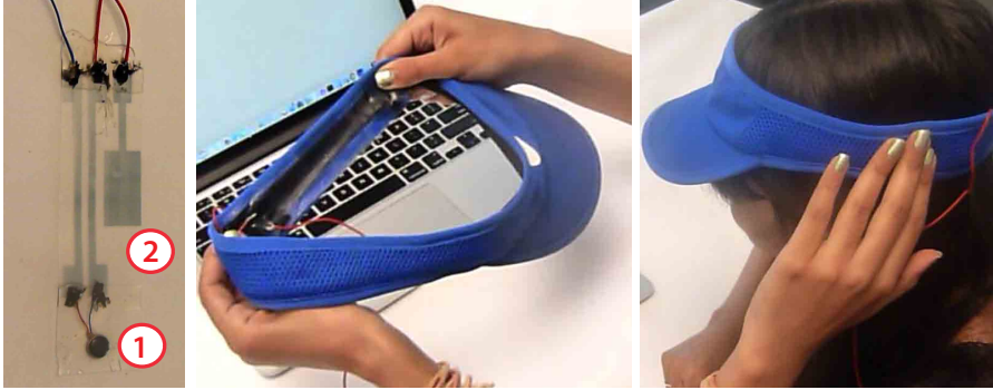
Figure 7: Interactive Head band. We integrated a stretchable touch/proximity sensor (1) and a vibration motor (2) into a stretchable head band. It notifies the wearer on incoming calls through vibration and the user can accept the call by touching the head band in proximity of the integrated sensor.
