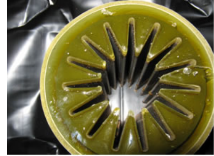
(b) Sub-scale motor propellant grain star geometry ©ONERA
