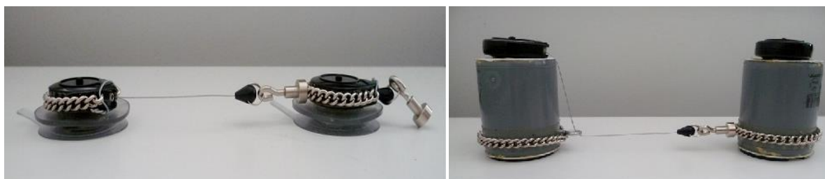
Figure 3.3. By attaching one Tangible Reel's retractable string to a Tangible Reel's metallic bracelet, a physical line can be built between two Tangible Reels. A strong neodymium magnet is attached at the end of each string.
