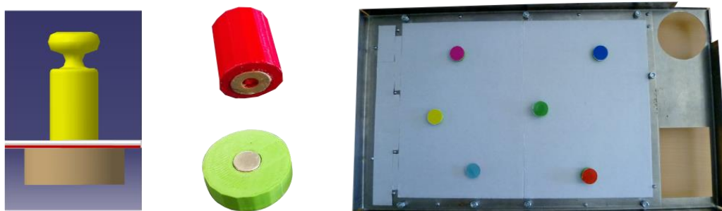
Figure 4.2. Each tangible object is composed of two parts, magnetically attached together. Left: the surface is between the two parts. Middle: 3D-printed objects with magnets inside. Right: view from below: a colored tag is affixed under the lower magnet for tracking and a magnetic sheet is glued (in white) to prevent an object from becoming detached.
