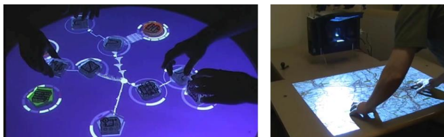
Figure 2.27. Two examples of camera-based systems. Left: with the ReactTable, the camera is placed below the surface (retrieved from [126]). Right: in PlayAnywhere, the camera is placed on the side of the table (retrieved from [341]).
