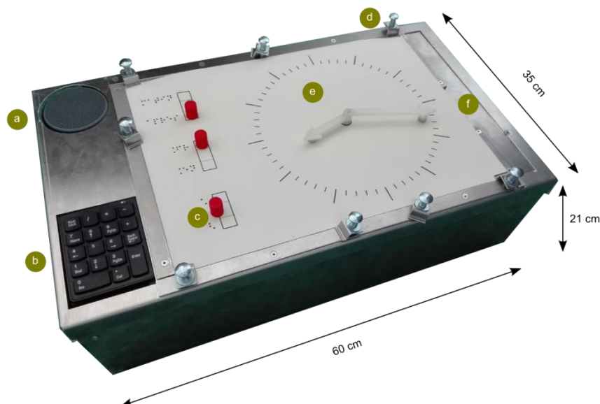
Figure 4.1. Overview of the Tangible Box. a) speaker; b) keyboard; c) a tangible object, composed of two parts (one above the surface, in red, and one below the surface); d) one element of the fastening system that holds the supports in place; e) support used for the activity (here, a raised-line clock); f) dedicated area where unused tangible objects can be placed.
