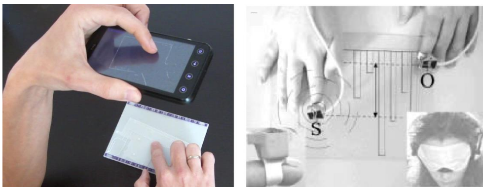
Figure 2.19. Two prototypes of interactive tactile maps with camera-based finger tracking. Left: in [85], users could interact with a 3D-printed map by holding their phone above it and the integrated camera tracked one of the user’s fingers (retrieved from [85]). With TouchMelody [247], two fingers were tracked to help users explore bar charts (retrieved from [247]).
