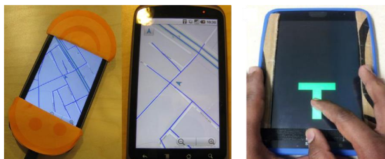
Figure 2.15. Two prototypes of digital maps with finger-based exploration. Left: TouchOverMap [241] allowed user to explore maps using vibrational and vocal feedback (retrieved from [241]). Right: in [79], vibrations and sounds indicated whether the user was touching vertices or edges (retrieved from [79]).
