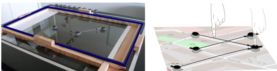
Figure 3.13. The system is composed of a transparent tabletop upon which an infrared frame (highlighted in blue, left) is placed to detect whenever the user performs a “tap and hold” gesture (right).
