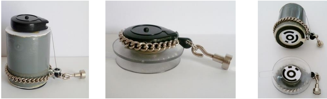
Figure 3.2. Final design of the two types of Tangible Reels. A Tangible Reel is composed of a retractable reel, a metallic bracelet and magnet. Left: Weights are composed of a plastic cylinder filled with lead; they are 6 cm high and 4 cm wide. Middle: Sucker pads are 2 cm high and 4 cm wide. Right: bottom view of the Tangible Reels with the TopCode tag visible.
