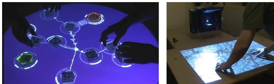
Figure 2.27. Two examples of camera-based systems. Left: with the ReacTable, the camera is placed below the surface (retrieved from [126]). Right: in PlayAnywhere, the camera is placed on the side of the table (retrieved from [341]).
