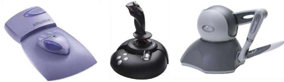
Figure 2.11. Three force-feedback input devices. Left: the Logitech Wingman mouse. Middle: the Microsoft Sidewinder joystick. Right: a Sensable Phantom device (now redistributed by Geomagic).
