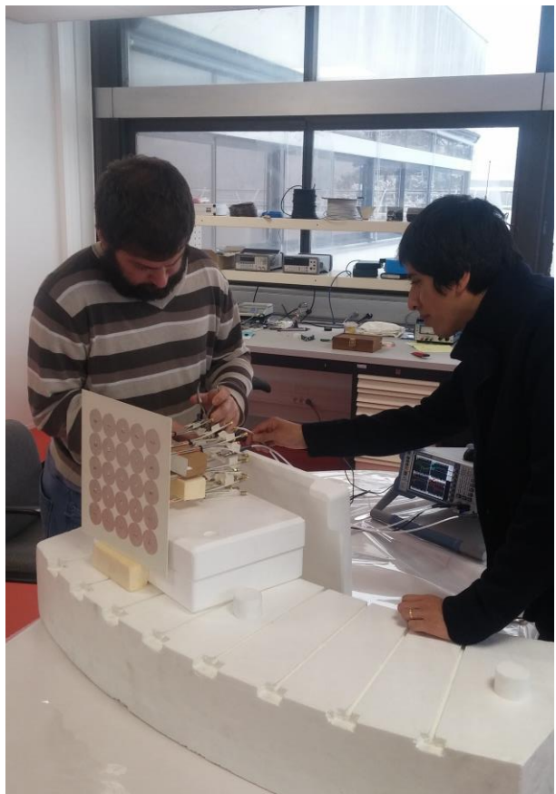
Fig. 3. 19 Measurement of the S parameters of the prototype array of 4 arms connecting non-complementary spirals.
