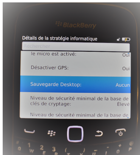
Figure 3.3: BlackBerry PGP Security Policy: Backup Unauthorised
