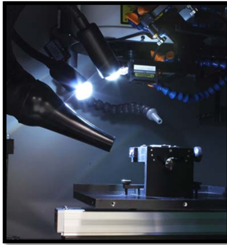
Figure 3.27: Ablation of Chip's Package by 1064 nm Laser
