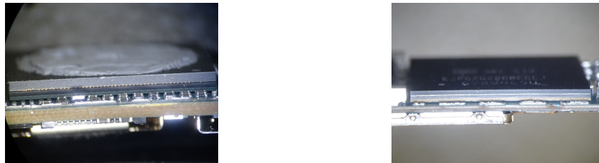
(a) BlackBerry Z10 PoP CPU: CPU (bottom) and RAM (top) (b) Samsung S7 edge: Qualcomm PoP processor
