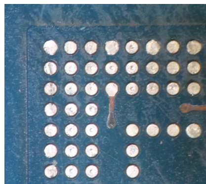
Figure 7.10: Donor Board eMMC Gap Position
