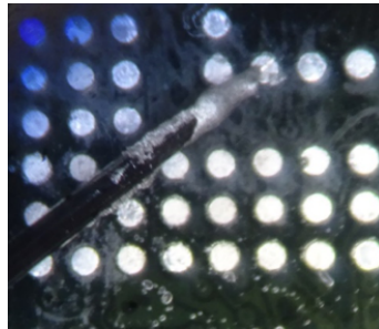
Figure 5.28: Step 3: Depositing ECA
