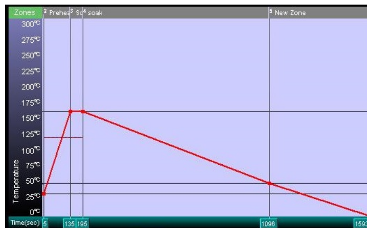
Figure 4.28: Slow Cooling ( 0.13\text{ }^{\circ}\text{C/s} ) Reflow Profile, X-axis (seconds), Y-axis (Celsius)
