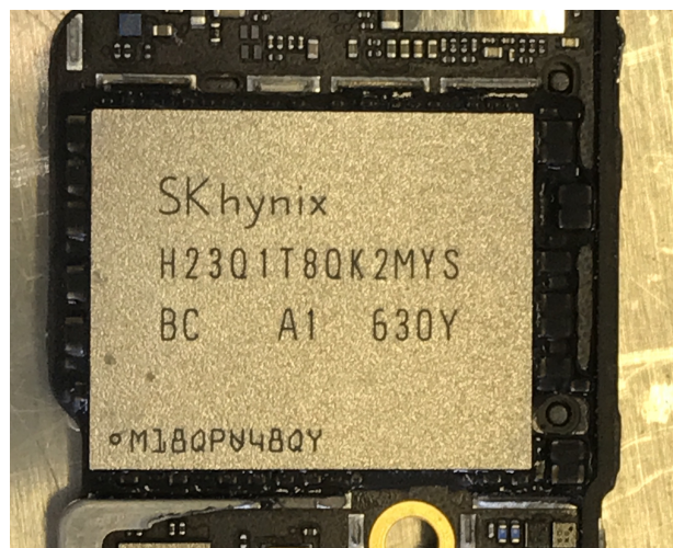
Figure 5.9: iPhone 7 Memory and Neighbourhood Capacitors Glued on Board
