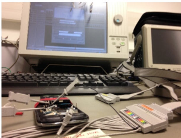
Figure 5.37: Tracking Signals Using a Logic Analyser or an FPGA
