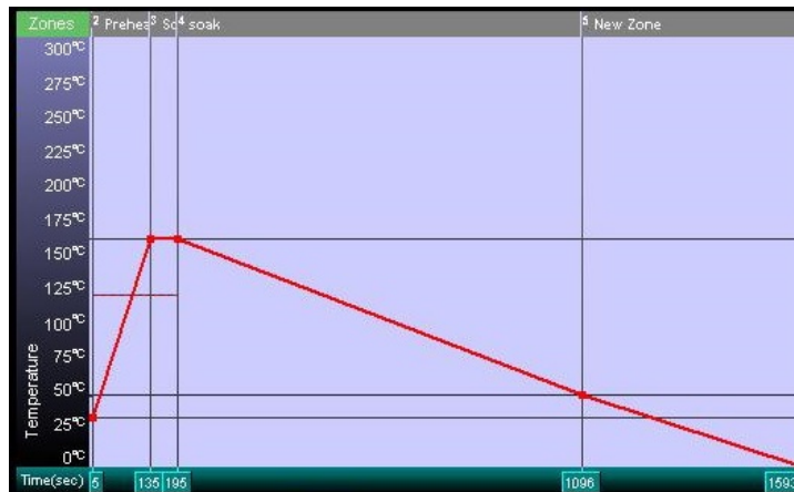
Figure 4.28: Slow Cooling ( 0.13\text{ }^{\circ}\text{C/s} ) Reflow Profile, X-axis (seconds), Y-axis (Celsius)
