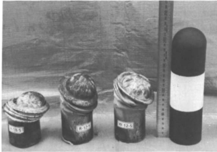
Figure 1.15: Kojima test missiles with different hardness (Kojima [79])
