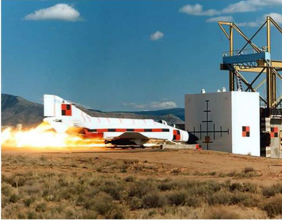
Figure 1.16: Full-scale aircraft impact test (Sugano et al. 182[129])
