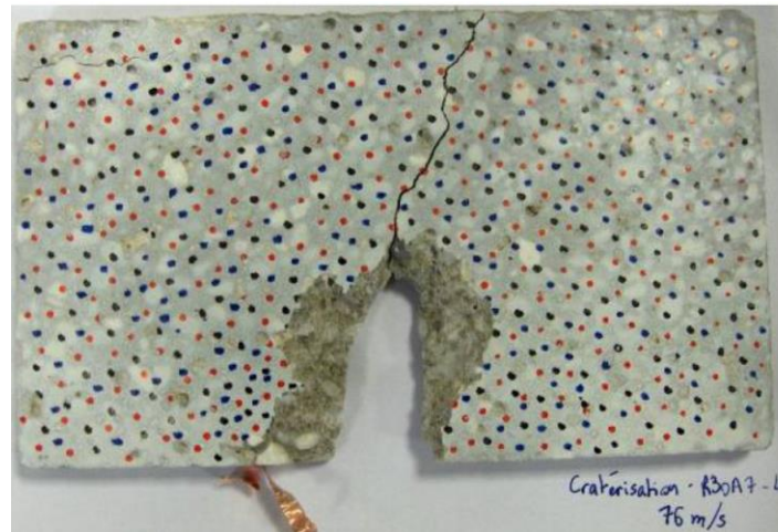
Figure 4.32: EOI-Small final damage state (experiment)
