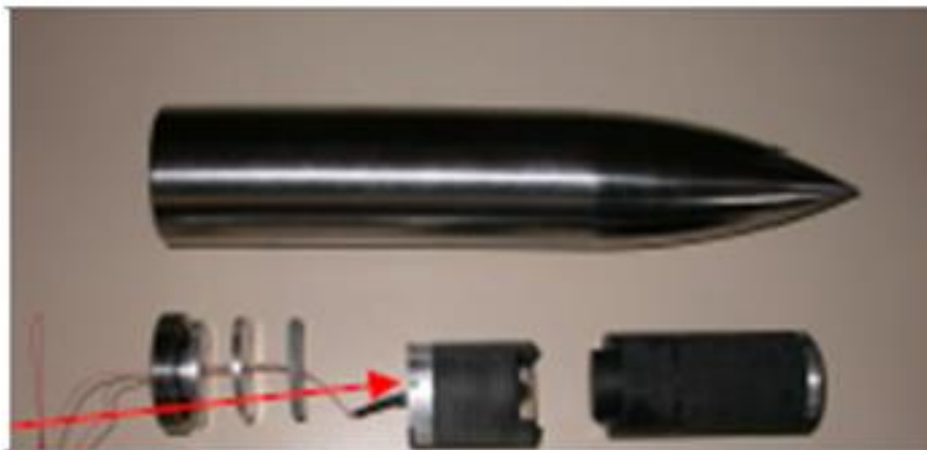
Figure 4.2: Ogive-nosed steel projectile with its accelerometer
