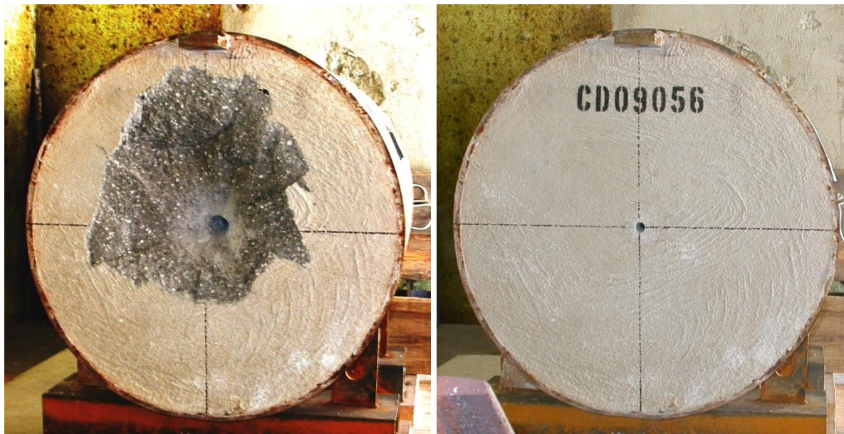
Figure 4.5: Target's front face (left) and rear face (right) after penetration LV test
