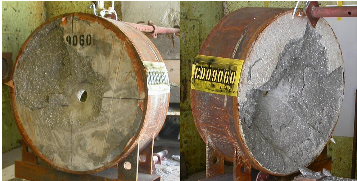
Figure 4.4: Target's front face (left) and rear face (right) after perforation test
