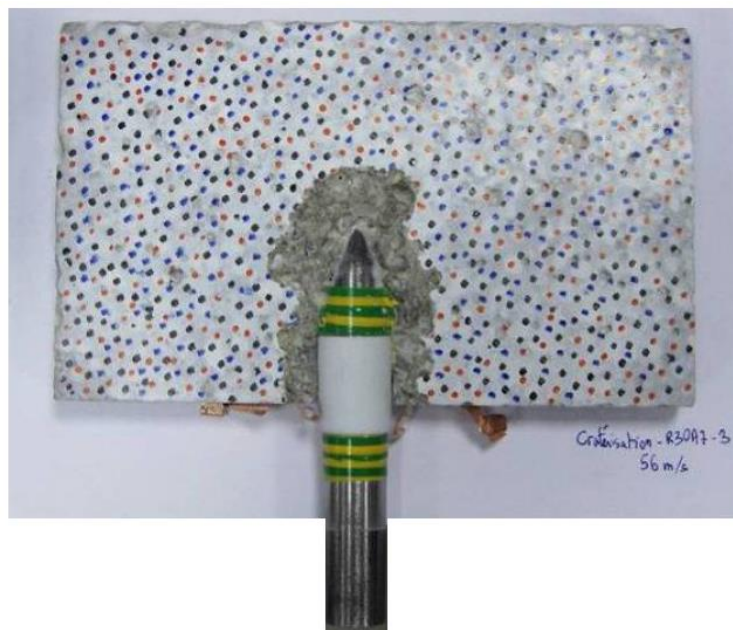
Figure 4.35: EOI-Big final damage state (experiment)
