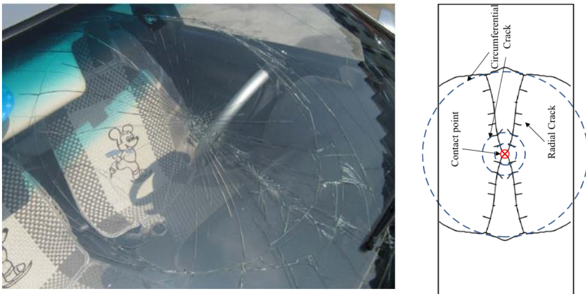
Figure 1.28: Cracks on windshield in real-world pedestrian-vehicle accident (left), simulation (right)
