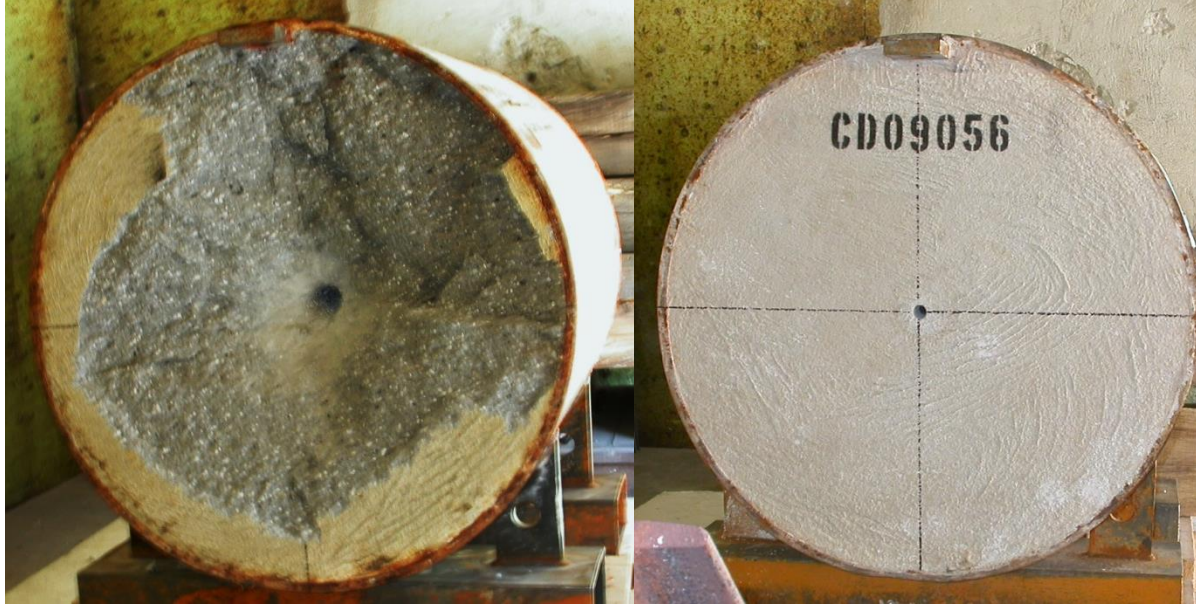
Figure 4.6: Target's front face (left) and rear face (right) after penetration HV test
