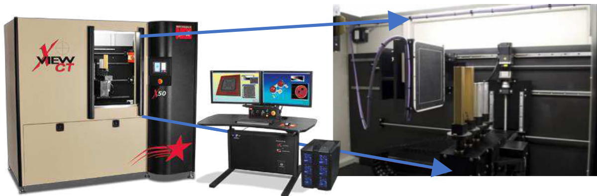
Figure 87. X-ray micro-tomographer available at ENS-Cahan (left); x-ray tube micro-oven of 225kV and detector of 3072x3888 pixels at high resolution (right). Adapted from [176].
