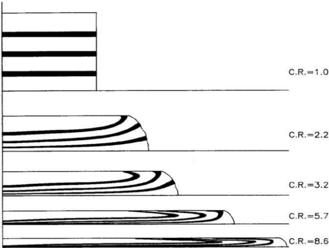
Figure 105. no-slip squeeze of a isothermal material for different compression ratio (C.R.) of a material with power-law index equal 0.3 [182]
