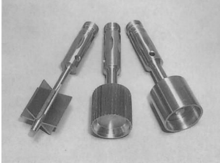
Figure 43. Haake viscometer SV geometries: vane with six-bladed (left), serrated cylinder (middle) and smooth cylinders (Right) [123].
