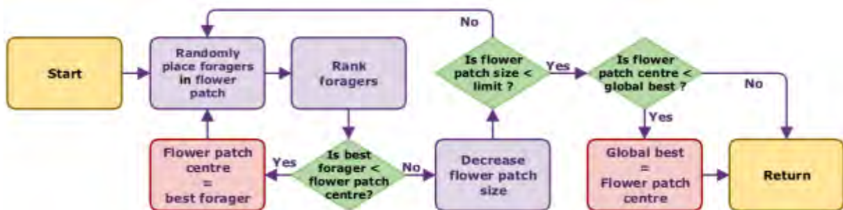
Figure 2.10: Schematic of a flower patch search. The forager bees are randomly located about a flower patch centre and then ranked. If any of the foragers are better than the flower patch centre, they replace it as the centre and then the process is repeated. If none of the foragers are better than the flower patch centre, the size of the flower patch is decreased and then the foragers are redistributed. Once the flower patch size shrinks beneath a certain limit, it is assumed that the local minimum has been found. This local minimum is compared to the best minimum that has been found so far by the algorithm (the global best). If it is better than the global best, it replaces it. The algorithm then moves on to searching the next flower patch.
