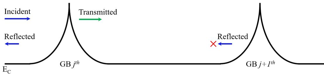
Figure 4.14: Schematic of the incident, reflected and transmitted electron waves in the conduction band at the  $j^{\text{th}}$  grain boundary.
