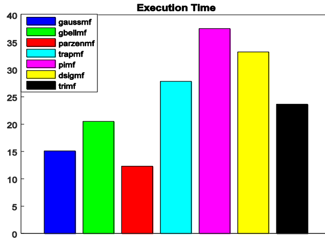
Figure 3.35: Graphical Representation of Consumption Time in Seconds for Different MFs (ANFIS Applied to Normal Reflux Rate Signal)
