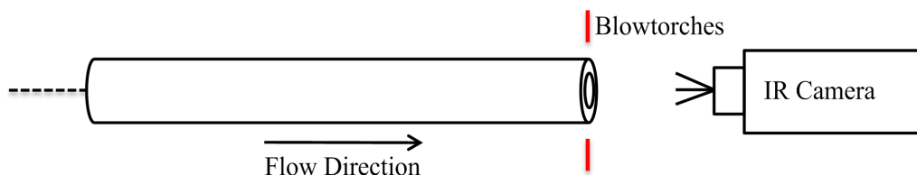
Figure 2.25: Schematic of the experimental layout.
