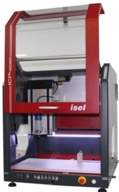
Fig. 2.5 Numerically controlled cutting machine “Fraiseuse”
