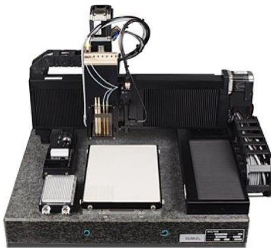
Figure IV-23: Machine de dispense SciFlex.
