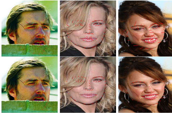
Fig. 2.5 Examples of prediction on LFPW test set. For visualizing errors, red segments have been drawn between ground truth and predicted landmark. Top row: MLP. Bottom row: MLP+in+out. (no unlabeled data)
