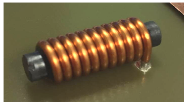
Figure 2.31: Application case: 2 \mu H inductor
