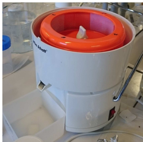
Figure 21: Centrifuge, where textile sample is placed on the edge of the tumble, used for draining most of water from textile fibres.
