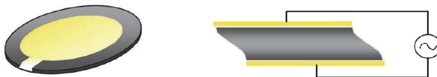
Figure 23 : Schematic representation of a gold-coated quartz crystal (left) and a cross section (right) of a deformed quartz crystal in grey with gold electrodes in yellow when an electric field is applied (picture adapted from Q-sense (Göteborg, Sweden) presentation of QCM).
