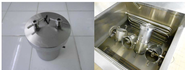
Figure 106 : (Left) sealed stainless steel container. (Right) stainless steel container placed on the rotated holder.
