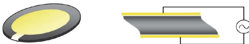
Figure 23 : Schematic representation of a gold-coated quartz crystal (left) and a cross section (right) of a deformed quartz crystal in grey with gold electrodes in yellow when an electric field is applied (picture adapted from Q-sense (Göteborg, Sweden) presentation of QCM).
