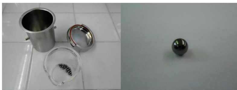
Figure 107 : (left) opened stainless steel container where the textiles and the stainless steel balls will be placed. (Right) Zoom on the stainless steel balls.
