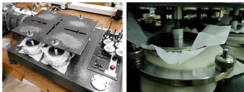
Figure 102 : (Left) Functionalised textiles placed against wool reps for abrasion test. (Right) zoom of the interface between the textile and the wool rep.
