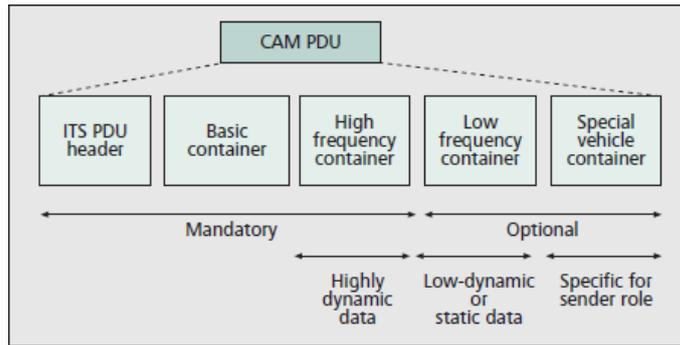
Figure 2.4: CAM structure (ETSI EN 302 637-2) [2, 3].
