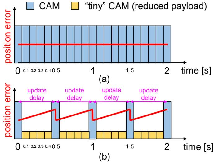
Figure 4.13: Standard CAM transmission policy (10 Hz) in (a) versus adjusted mixed CAM traffic (including tiny/frequent CAMs at 10 Hz and nominal/infrequent CAMs at 2 Hz) in (b).
