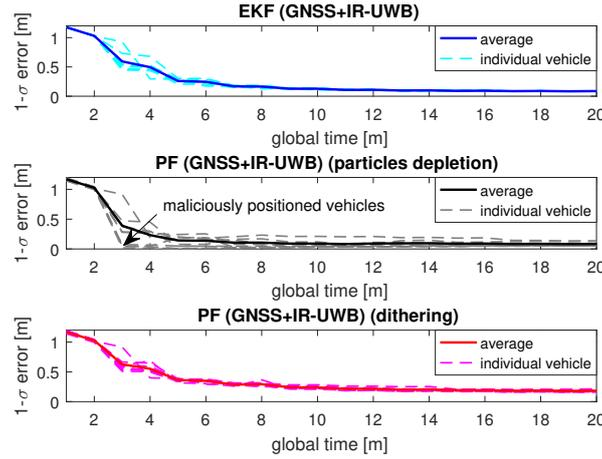
Figure 5.13:  $1-\sigma$  estimation errors perceived by fusion filters for each vehicle during the first 2 seconds for the fused GNSS+IR-UWB ranges using EKF (top), conventional PF (middle), and PF with adaptive dithering (bottom).
