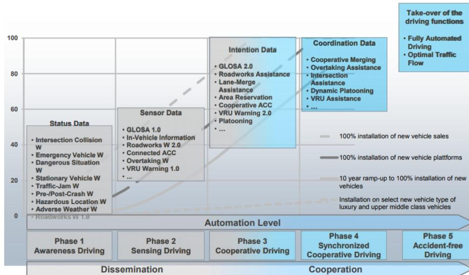
Figure 2.2: The C2C-CC applications road map (Source: C2C-CC).
