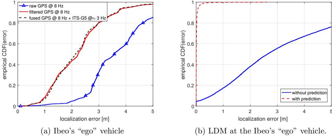
Figure 7.8: Empirical CDFs of localization errors for the first trip of field trials in Helmond.
