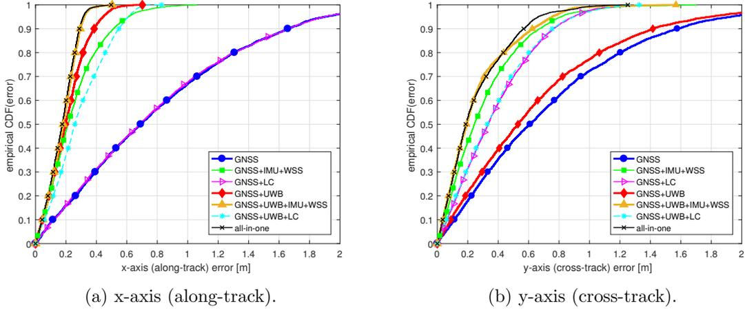
Figure 6.5: Empirical CDFs of x-axis (along-track/left) and y-axis (cross-track/right) localization errors for different fusion schemes in the two-lane highway scenario.
