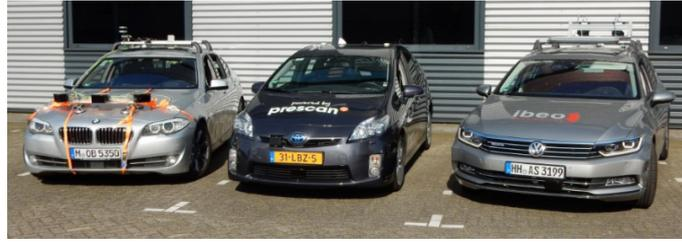
Figure 7.5: Test vehicles involved in the first HIGHTS field trials carried out in Helmond: Objective’s BMW, Tass’s Prius and Ibeo’s Passat (left to right).
