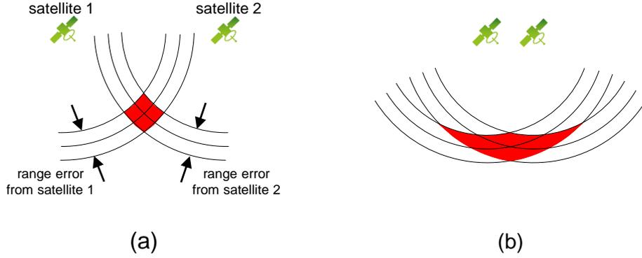
Figure 2.5: Effect of DOP in satellite-based positioning systems.
