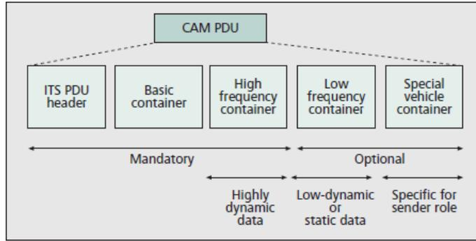
Figure 2.4: CAM structure (ETSI EN 302 637-2) [10, 21].
