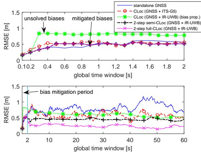
Figure 5.9: Localization RMSEs considering degraded GNSS vehicles as a function of time for different PF fusion schemes and different measurements/technologies for the mitigation of filter overconfidence and error propagation.
