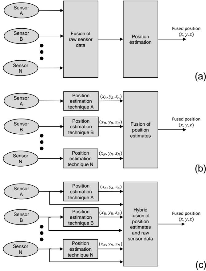
Figure D.1: Generic fusion architectures: (a) centralized (low-level), (b) autonomous (high-level), (c) hybrid (partial reproduction and simplification of [1]).
