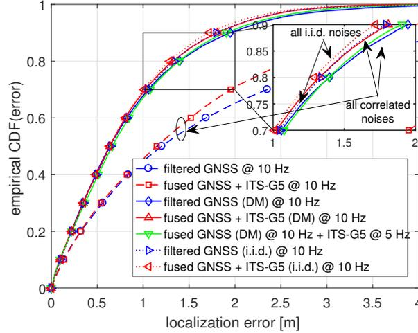
Figure 4.11: Localization performance comparison of different schemes assuming correlated GNSS noise and correlated shadowing, except the two dotted curves corresponding to both i.i.d. GNSS noise and RSSI shadowing cases in the urban canyon scenario.
