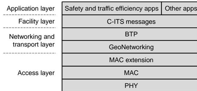
Figure 2.3: The C-ITS protocol stack (partial reproduction of [8, 10]).
