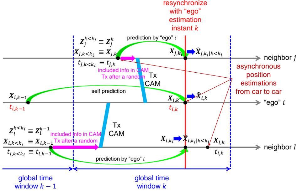
Figure 3.2: Example of space-time schematic managed by the “ego”  $i$  whose neighbors are vehicles  $j$  and  $l$ . Due to asynchronous estimates, the “ego”  $i$  needs to perform prediction of received information at its time of interest  $t_{i,k}$ .
