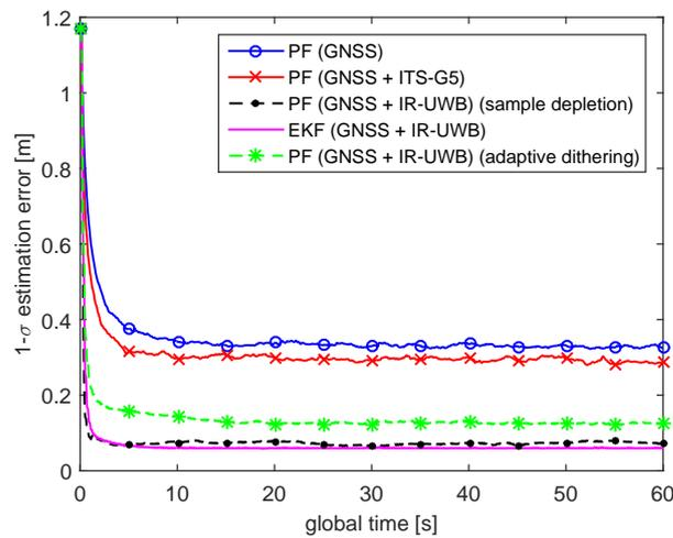
Figure 5.12: Average  $1\text{-}\sigma$  estimation errors perceived by fusion filters for different fusion techniques, schemes, and measurements/technologies for the mitigation of filter overconfidence and error propagation (including accurate V2V range measurements).
