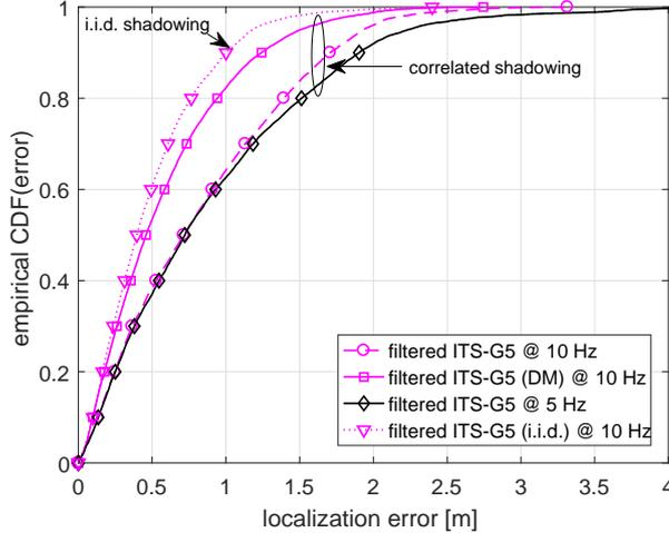
Figure 4.12: Localization performance comparison of different schemes assuming loss of GNSS signal and correlated shadowing, except the top curve corresponding to i.i.d. RSSI shadowing case in the tunnel scenario.
