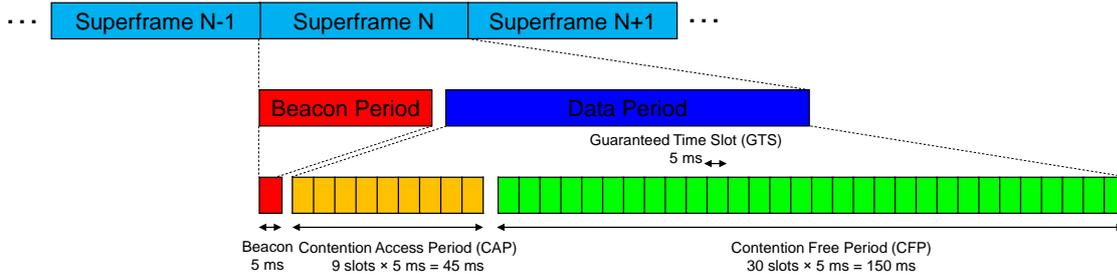
Figure 5.2: Beacon-aided TDMA MAC SF format supporting the localization functionality (SF duration of 200 ms).
