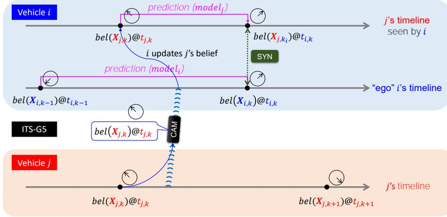
Figure 3.3: Example of CLoc space-time data management at the “ego” vehicle  $i$  with respect to its neighboring vehicle  $j$ . Due to asynchronous sampled time instants  $t_{i,k} \neq t_{j,k}$ , vehicle  $i$  needs to perform a prediction of the received information i.e.,  $bel(\mathbf{X}_{j,k})$  at any fusion time of interest  $t_{i,k}$  i.e.,  $bel(\mathbf{X}_{j,k_i})$ .
