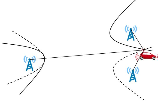
Figure C.3: 2-D localization based on TDOA measurements.
