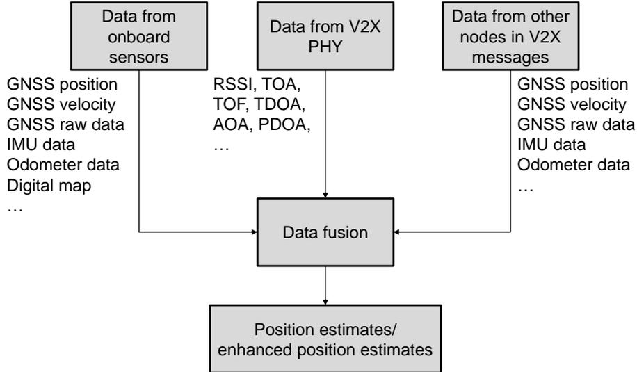
Figure 2.7: Dataflow of CLoc in an “ego” vehicle.
