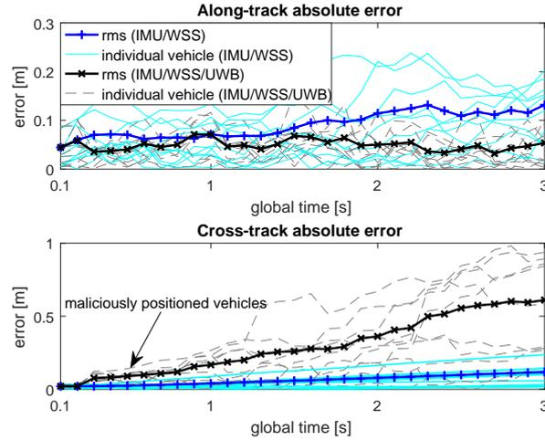
Figure 6.2:  $1\text{-}\sigma$  along-track (top) and cross-track (bottom) errors perceived by fusion filters for each vehicle during the first 3 seconds for non-CLoc (IMU/WSS) and pure CLoc (IMU/WSS/UWB) in a tunnel scenario. Simulation settings and scenarios are given in Section 6.5.
