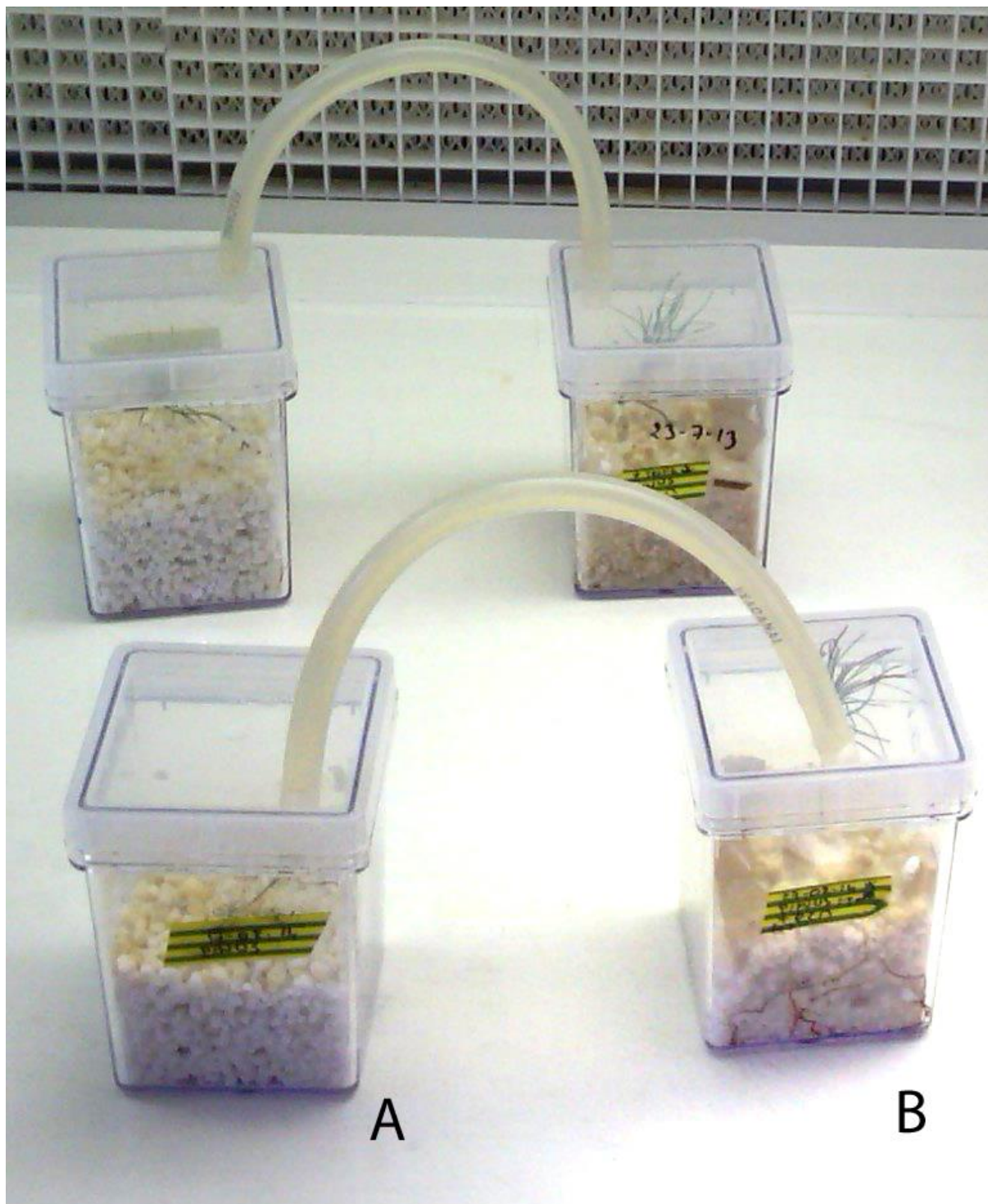
FIGURE S1. Experimental design to measure the potential EM fungal respiration and ^{13}\text{CO}_2 transfer in a Magenta box. A. Magenta box with a non-mycorrhizized seedling (Scots pine), without P. placenta necromass. B. Magenta box with a mycorrhizized seedling, with P. placenta labelled necromass. Boxes were connected with a flexible and hermetic tube.
