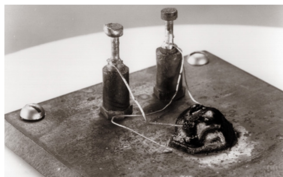
Figure 1. Left: John Bardeen, William Shockley and Walter Brattain. Right: the first point-contact transistor
