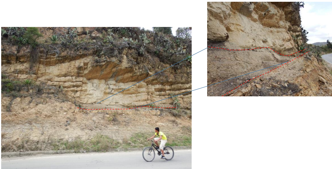
Photo 3.5. Outcrop of the Churuvita Formation along the Sachica road, before the deviation towards Cucaita –Villa de Leyva town. Note the unconformity with a possible level of paleosol at the base, overlaid by thick, to medium-grained, white to yellow sandstone beds.
