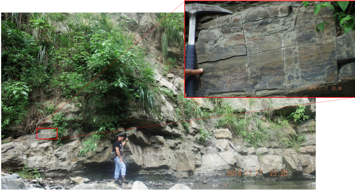
Photo 3.1. Litharenite of Early Aptian age (Upper Trinchera Fm). Note the lens-shaped layers and cross laminations (upper red square).
