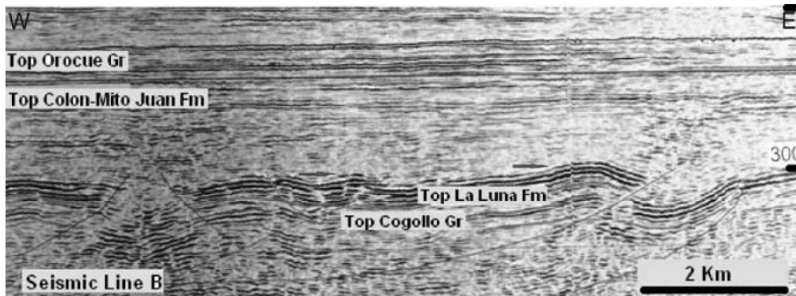
Figure 4.28. Seismic profile in the Maracaibo Basin (Venezuela), flattened on the horizon "Colon-Mito Juan" units (Cooney and Lorente, 2012). Note the compressional deformation of pre-Late Campanian age.
