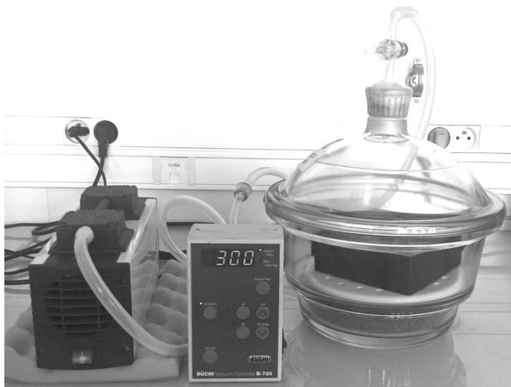
Figure 3.8 – Device developed in the laboratory to dehydrate aqueous GO dispersions. From the left to the right: vacuum pump, pressure controller and vacuum chamber.
