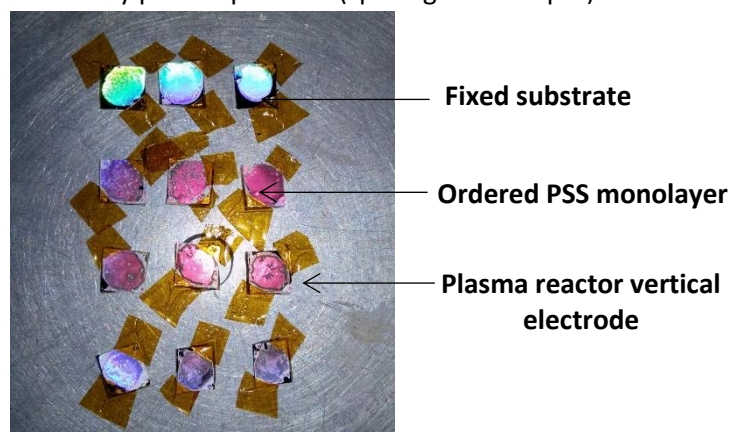
Fig. IV - 7 : Image of substrates with PS self-assembled spheres fixed to one electrode for plasma etching (vertical electrodes).
