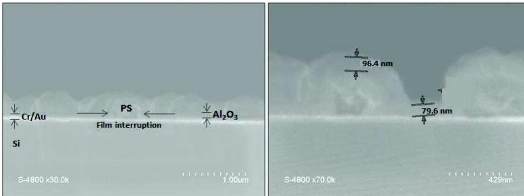
Fig. V - 12 : SEM images of a cross-sectioned region for a 60 nm  $\text{Al}_2\text{O}_3$  covered PS sample. Right image is a zoom around the particle of left image that shows an interruption of  $\text{Al}_2\text{O}_3$  film.
