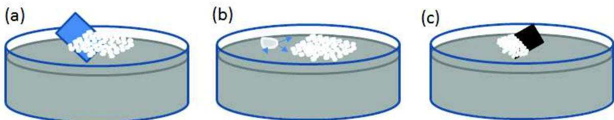
Fig. IV - 4 : PSS deposition process, a. insertion of glass substrates with the solution of PSS (white spheres) organizing on the air-water interface; b. addition of SDS drop, and c. transfer on substrates of PSS monolayer.
