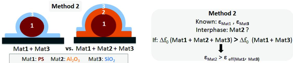
Fig. V - 39: Interphase detection method 2, left: sketch of the samples to be compared, right: methodology.
