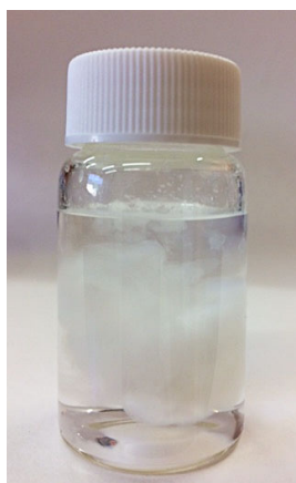
Figure 36. Photograph of the film obtained incorporating 100 mol. % of citric acid into the WNIPU4 dispersion after immersion in water.
