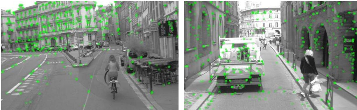
Figure 6-19 ORB-SLAM image processing (Test 1)
