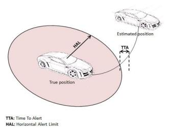
Figure 5-1 Loss of integrity
