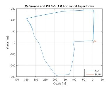
Figure 6-22 Comparison between ORB-SLAM and reference trajectories (Test 1)
