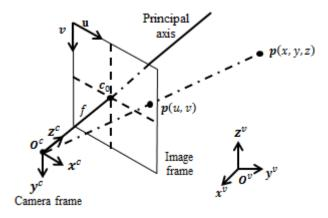
Figure A-3 Image, camera and vision frames
