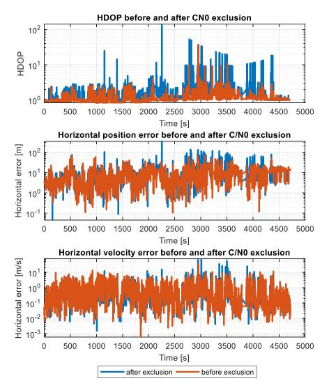
Figure 6-11 Impact of the low  $C/N_0$  exclusion on HDOP, horizontal position error and horizontal velocity error in suburban-urban environment
