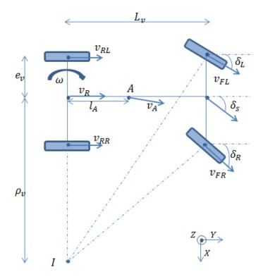
Figure 2-6 2D Ackermann steering model
