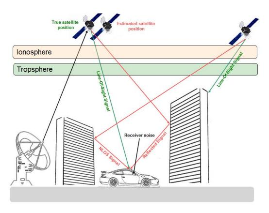
Figure 2-1 GNSS error sources
