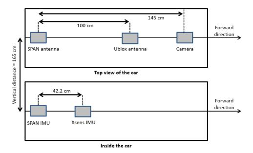
Figure 6-4 Sensor configuration for data collection
