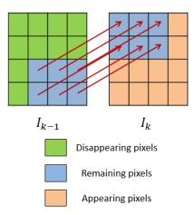
Figure 3-5 Optical flow matching
