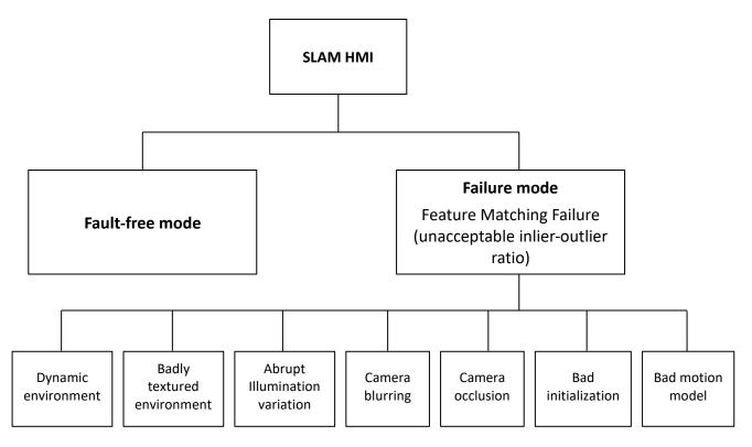
Figure 5-4 VSLAM fault tree
