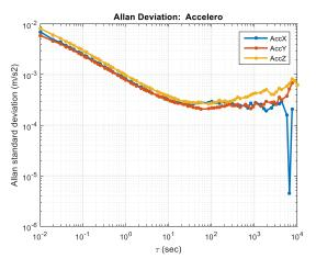
Figure 2-3 Allan variance deviation of the IMU accelerometers
