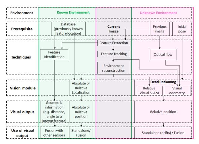
Figure 3-1 Classification of vision-based techniques
