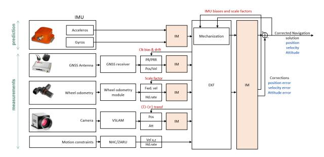
Figure 5-6 multi-sensor architecture integrity monitoring
