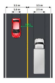
Figure 5-5 HAL computation from a typical traffic example
