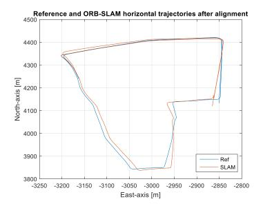
Figure 6-23 Reference and ORB-SLAM trajectories after alignment (Test 1)
