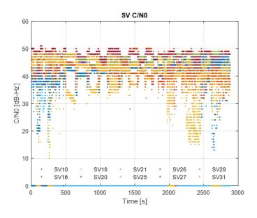
Figure 6-14  $C/N_0$  of GPS measurements in airport environment
