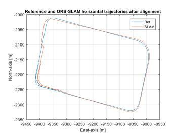
Figure 6-27 Reference and ORB-SLAM trajectories after alignment (Test 2)
