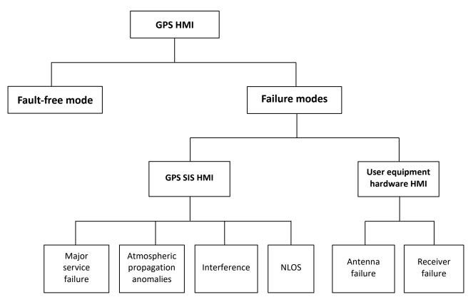
Figure 5-3 GPS fault tree
