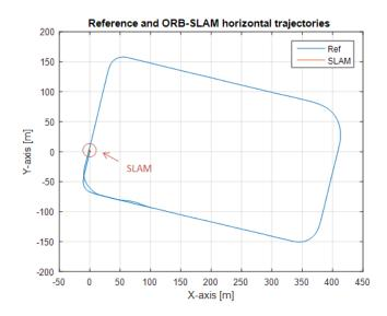
Figure 6-26 Comparison between ORB-SLAM and reference trajectories (Test 2)
