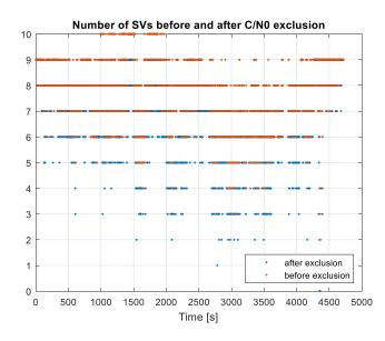
Figure 6-10 Number of GPS measurements before and after exclusion through comparison to  $C/N_0 = 30$  dB-Hz in suburban-urban environment
