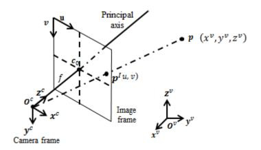
Figure 3-3 Pinhole camera projection
