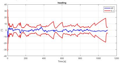
Figure 6-31 Heading error and its associated  $3\sigma$  bound of the GPS/INS/WSS/NHC filter (Test 1)
