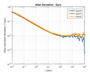
Figure 2-2 Allan variance deviation of the IMU gyroscopes
