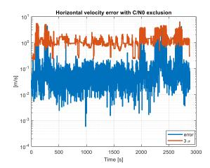
Figure 6-17 GPS L1 horizontal velocity error and its associated  $3\sigma$  bound with low  $C/N_0$  exclusion in airport environment
