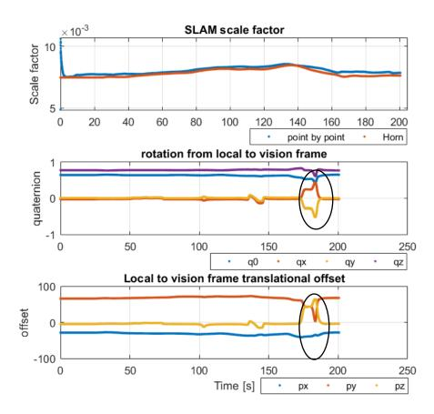
Figure 6-28 ORB-SLAM transformation estimation (Test 2)
