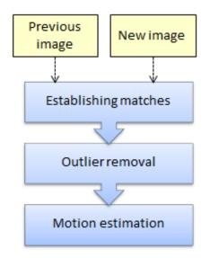
Figure 3-4 Visual odometry diagram
