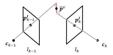
Figure 3-8 VSLAM triangulation process
