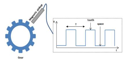
Figure 2-5 Principle of the magnetic WSS
