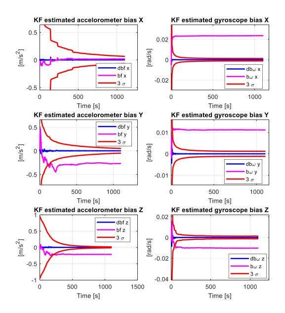
Figure 6-32 IMU accelerometer and gyroscope biases and their associated  $3\sigma$  bound of the GPS/INS/WSS/NHC filter (Test 1)
