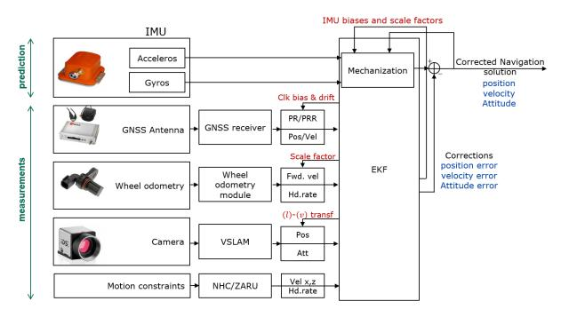
Figure 4-1 Multi-sensor fusion architecture
