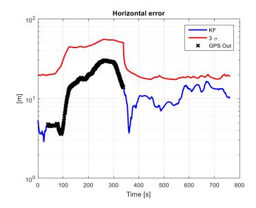
Figure 6-38 Horizontal position error and its associated 3σ bound of the GPS/INS/WSS/NHC/IT/VSLAM filter with 300 s GPS outage (Test 1)
