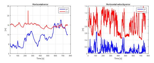
Figure 6-36 Horizontal position and velocity errors and their associated  $3\sigma$  bound of the GPS/INS/WSS/NHC/IT/VSLAM filter (Test 1)
