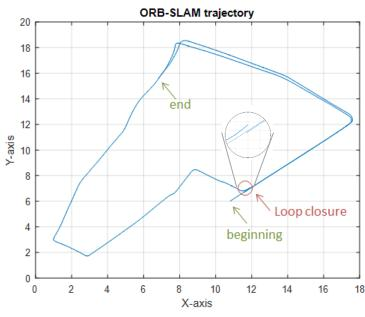
Figure 6-18 ORB-SLAM trajectory in vision frame (Test 1)
