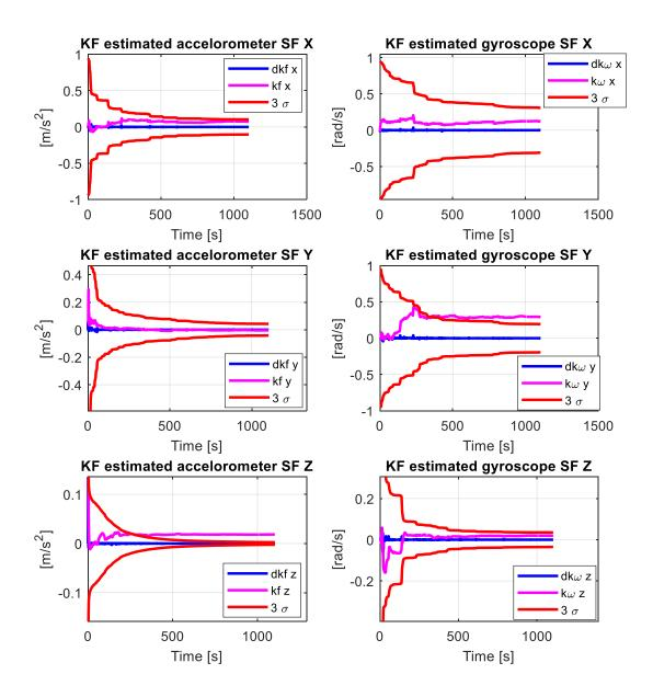
Figure 6-33 IMU accelerometer and gyroscope scale factors and their associated  $3\sigma$  bound of the GPS/INS/WSS/NHC filter (Test 1)
