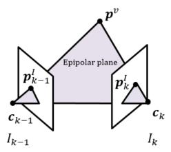
Figure 3-7 Epipolar geometry constraint
