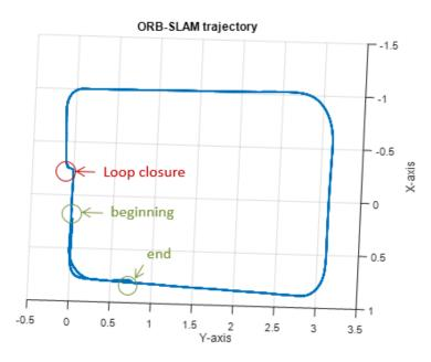
Figure 6-21 ORB-SLAM trajectory in vision frame (Test 2)
