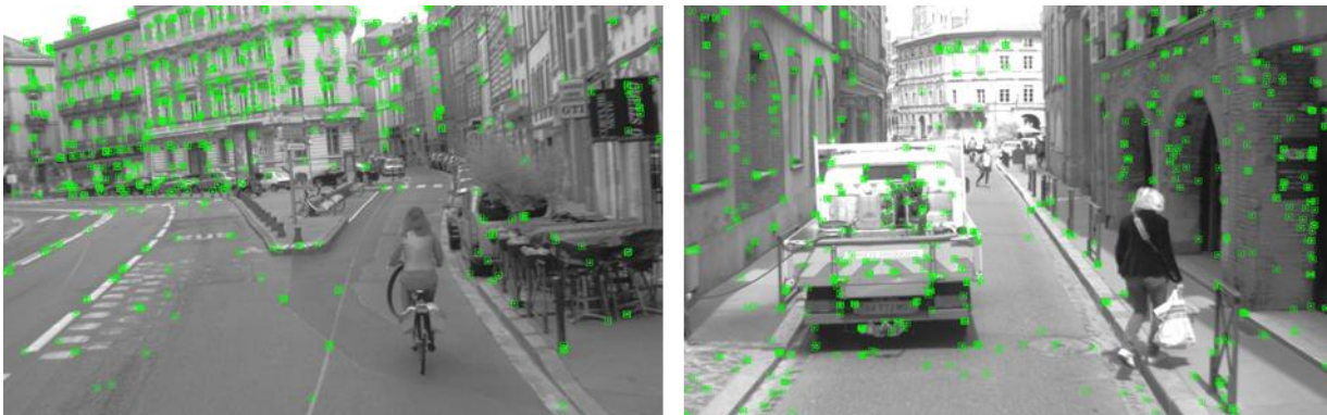
Figure 6-19 ORB-SLAM image processing (Test 1)
