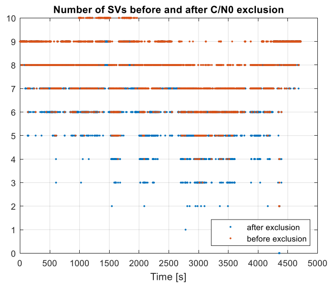
Figure 6-10 Number of GPS measurements before and after exclusion through comparison to C/N_0 = 30 dB-Hz in suburban-urban environment
