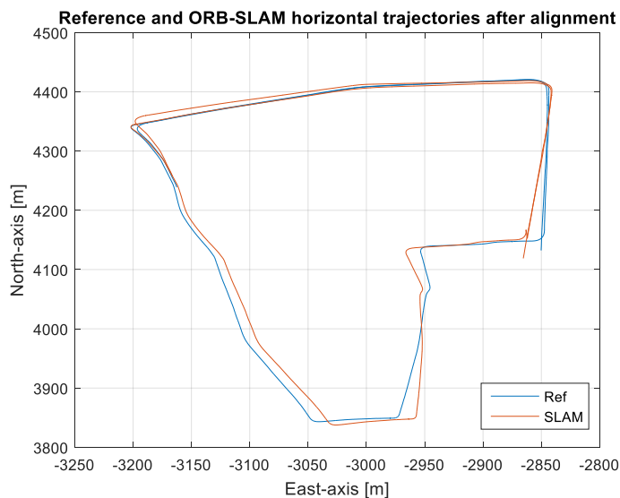
Figure 6-23 Reference and ORB-SLAM trajectories after alignment (Test 1)
