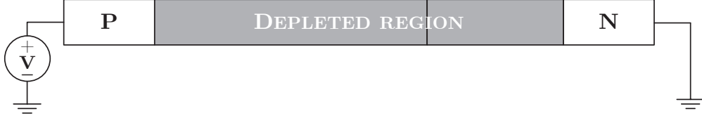
Figure 2.8: Polarized pn junction
