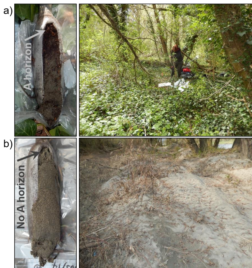
Figure VII-7: a) Example of pre-dam surface conditions (DZM reach). Left: Surface sample from a sampling plot centre. Right: ground surface conditions in the same plot. b) Example of post-dam surface conditions (MON reach). Left: Surface sample from a sampling plot centre. Right: ground surface conditions in the same dike field. All four photos were taken in the course of two days in mid-March 2014.
