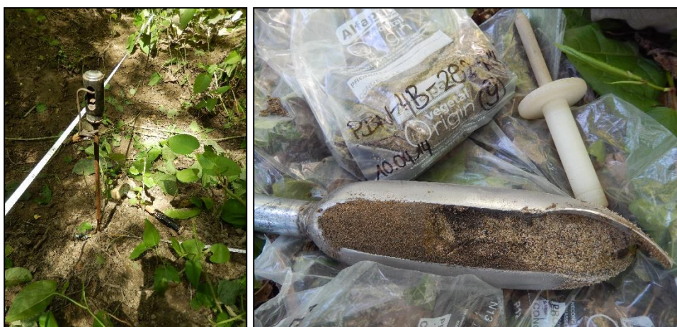
Figure III-10: Use of the iron rod to determine overbank fine sediment thickness (left). Overbank fine sediment sample extracted using the soil auger (right).
