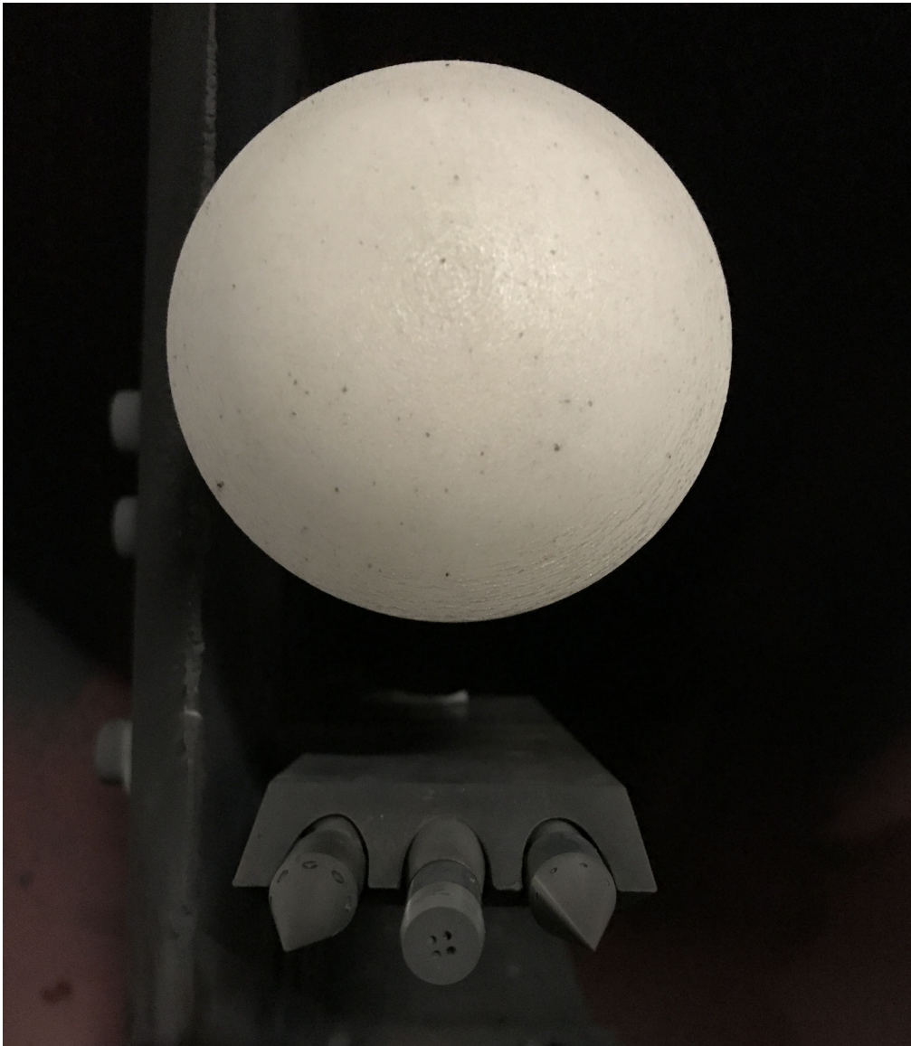
Figure 4.11: Photo of the second iteration of the standalone Pitot probe mount model mounted underneath a 3D printed scaled Hayabusa test model.
