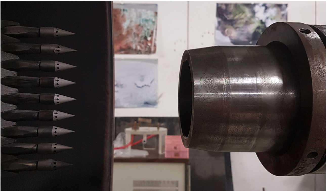
Figure 4.9: X2's Pitot rake during experimental set up to measure pressures at the same axial location as the entrance to X2's nozzle from McLean [245].
