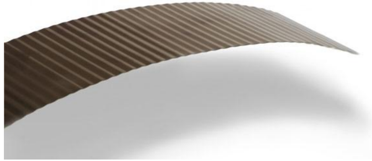
Figure 3.1: Corrugated ribbon damper
