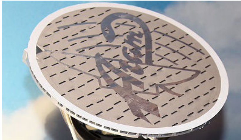
Figure 1.7: 9B-1103M Russian active radar seeker antenna
