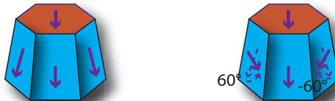
Polarisation purity and ellipticity remain much higher when the lateral elements remain vertical
