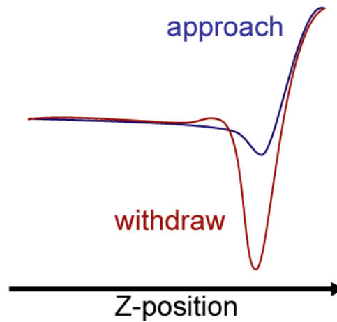
Figure 1.10 – Typical force curve: approach (blue) and withdraw (red) versus piezo Z (vertical) position. Source: Peak Force QNM User Guide [43].
