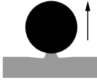
Figure 2.3 – Formation of an adhesive neck when the surfaces separate, as predicted by the JKR contact model.
