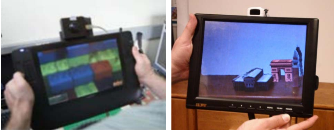
Figure 2.5 – Handheld displays are mainly used for AR purposes. Devices have been proposed by Hill et al. [2011] (left) and Baricevic et al. [2012] (right) to display a coherent viewpoint when using handheld displays.
