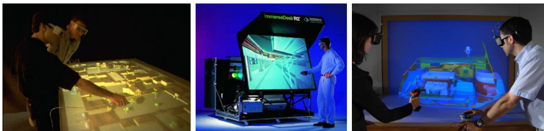
Figure 2.7 – Examples of workbench displays: the Responsive Workbench [Krüger et al., 1995] (left), the Immersadesk [Czernuszenko et al., 1997] (middle) and a Holobench from PSA Peugeot Citroën (right).
