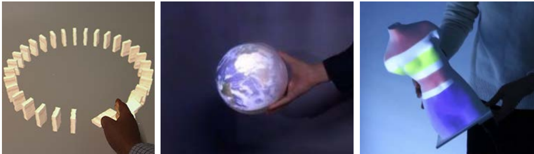
Figure 2.10 – Examples of spatial augmented reality displays: The Mirage Table from Benko et al. [2012] (left), the Lumipen from Okumura et al. [2012] (middle) and the Pmomo approach from Zhou et al. [2016] (right).
