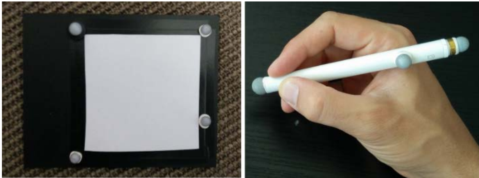
Figure 5.7 – Tangible interaction tools of MoSART: the interactive Panel (left) and the interactive Stylus (right).
