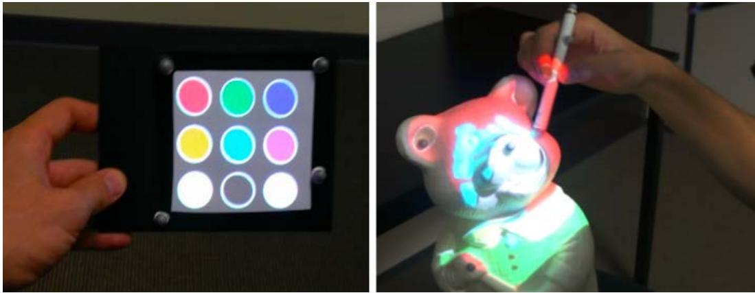
Figure 5.10 – Virtual painting. The user can select a color on the Panel (left) and paint the tangible object with the Stylus (right).
