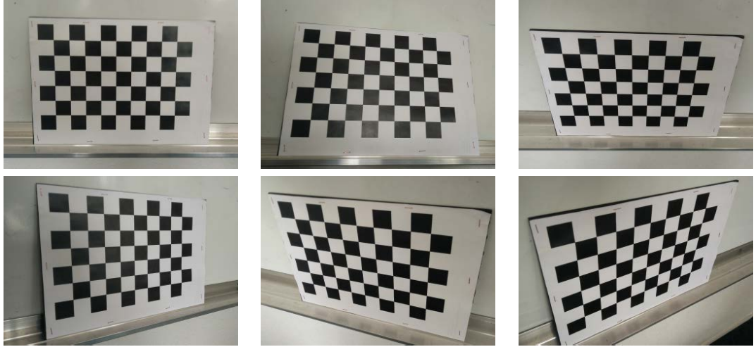
Figure 4.7 – During the internal camera calibration process, several views of a chessboard are captured and 2D features are extracted to compute the internal parameters of the cameras.
