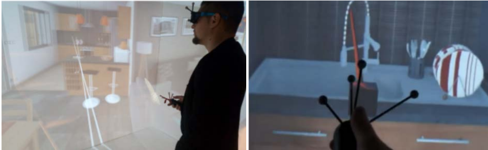
Figure 3.2 – Our pilot study VR application in use: a user interacting in the CAVE display (left) and a first-person view during the selection an object made with a virtual ray controlled by the Wand device (right).
