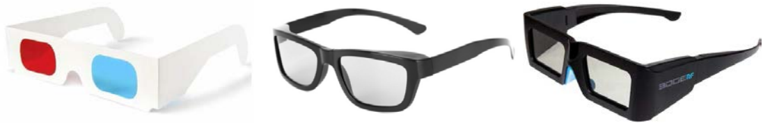
Figure 2.6 – Examples of stereoscopic glasses: Anaglyphic stereo glasses that use spectral filters (left), polarized stereo glasses that use polarized filters (middle) and active stereo glasses that work with shutters (right).
