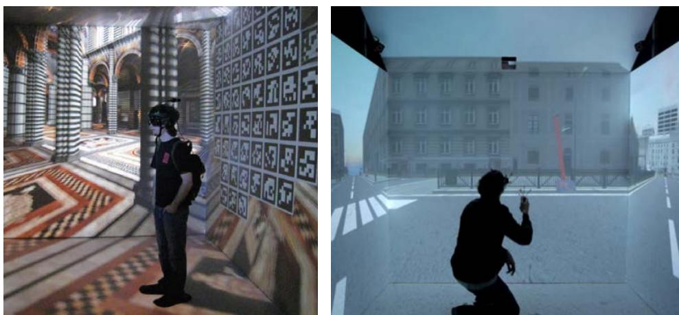
Figure 2.23 – Examples of tracking techniques used in surround screen displays environments: JanusVF Inside-out tracking [ Hutson and Reiners, 2011 ] (left) and an outside-in infrared optical tracking from Realyz (right).
