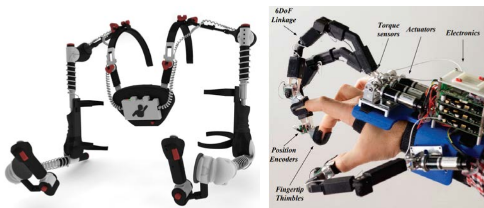
Figure 2.13 – Examples of mechanical tracking systems: Gypsy's upper body exoskeleton (left) and the HEXOTRAC hand mechanical exoskeleton [Sarakoglou et al., 2016] (right).
