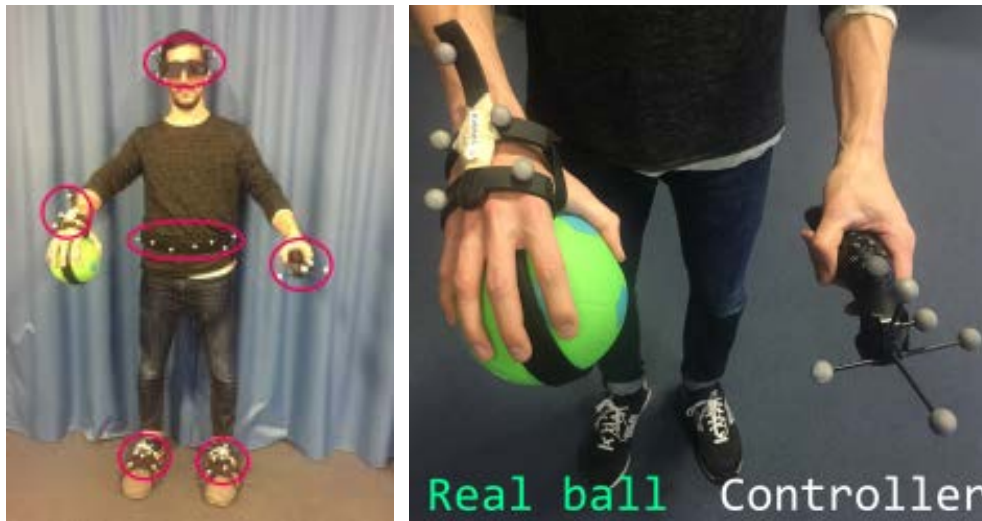
Figure 6.2 – Six infrared constellations (red) were placed over the participants (left) to provide tracking data to perform the inverse kinematics optimization. A ball was placed in their right hand, as an extension of their arm, and a controller in their left one (right).
