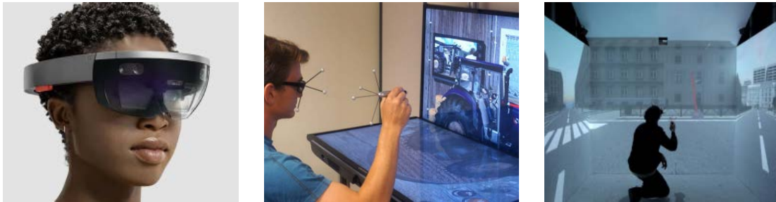
Figure 1.3 – Examples of mixed reality displays: the Microsoft HoloLens near-eye display (left), an Holobench screen display from Realyz (middle) and a CAVE projection-based system from Realyz inspired by Cruz-Neira et al. [1993] (right).
