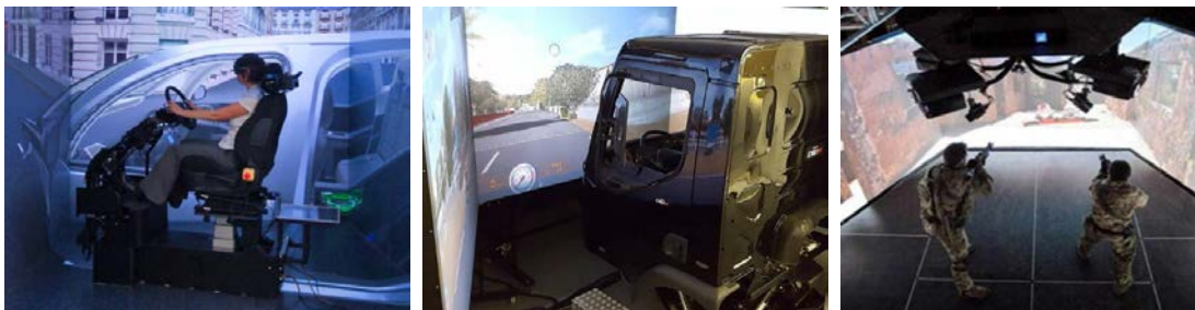
Figure 2.25 – Mixed Reality training applications for the industry: the PSA Citröen projection-based VR driving simulator (left), the Thales truck driving simulator (middle) and the VirTra simulator for police officer training in real life conditions (right).
