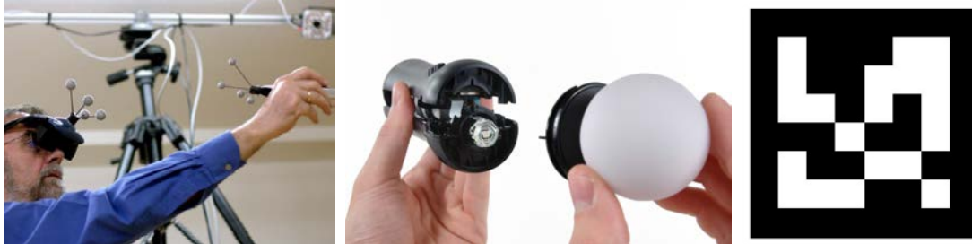
Figure 2.19 – Examples of markers used in optical tracking devices: passive markers used by Pintaric and Kaufmann [2007] (left), active colored markers used in the PSMove device from Sony (middle) and a squared fiducial marker [ Hutson and Reiners, 2011 ] (right).
