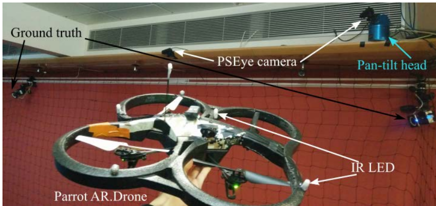
Figure 4.20 – Our optical tracking approach for UAV localization and for comparison with Vicon's optical tracking system.
