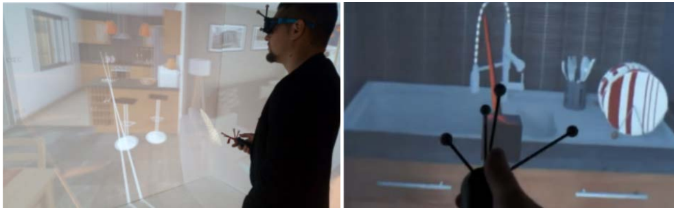
Figure 3.2 – Our pilot study VR application in use: a user interacting in the CAVE display (left) and a first-person view during the selection an object made with a virtual ray controlled by the Wand device (right).
