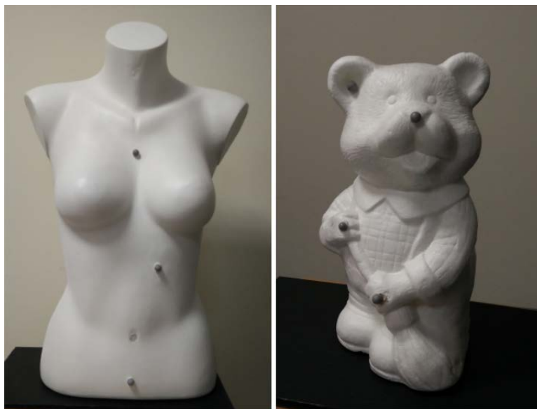
Figure 5.4 – Example of tangible objects augmented with MoSART. The objects are white or covered with white painting. Reflective markers are positioned over the objects to facilitate their localization.
