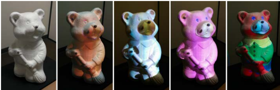
Figure 5.9 – Several textures can be applied to an object for virtual prototyping purpose. The original teddy bear tangible object (left) is augmented with various textures selected on the interactive Panel.
