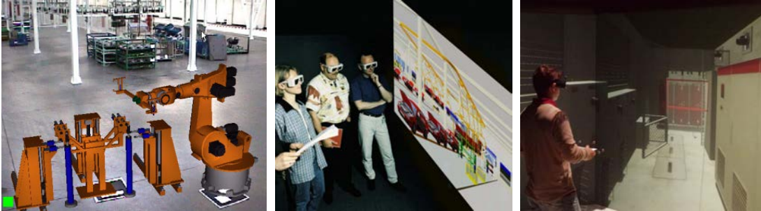
Figure 2.28 – Planning applications of Mixed Reality in the industry: an AR planning application for factory layout [Doil et al., 2003] (left), a project team validating the planned manufacturing system [Dangelmaier et al., 2005] (middle) and the validation of a solar plant in a CAVE environment [Medeiros et al., 2013] (right).
