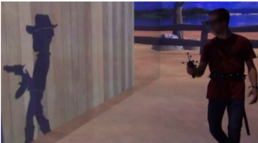
Figure 7.1 – Virtual embodiment through virtual shadows in an entertainment VR application – The virtual shadow of a cowboy (Inspired from the famous Lucky Luke comic book) is displayed in a far west virtual scene in a CAVE display.
