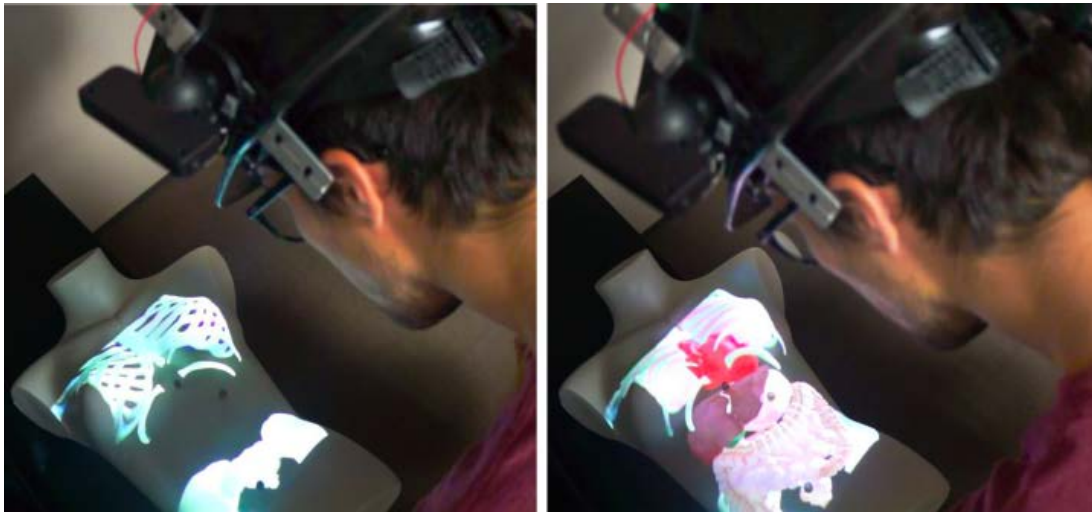
Figure 5.11 – Medical visualization on a tangible chest with MoSART. The user is able to visualize the bones (left) with or without the organs (right).
