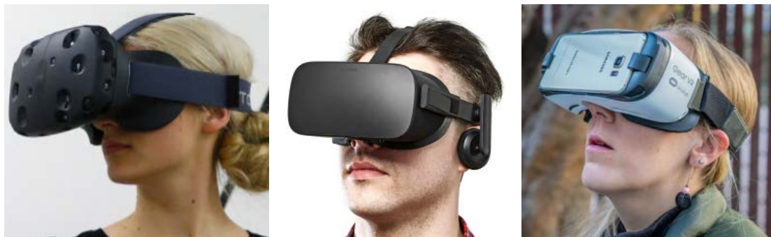
Figure 2.2 – Examples of non see-through HMD used for VR applications: the HTC Vive (left), the Oculus Rift (middle) and the Samsung Gear VR which relies on a smartphone (right).
