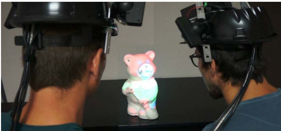
Figure 5.13 – Concept of a collaborative setup with two MoSART systems (photomontage). The users could look at different sides of the object for an even wider projection space.
