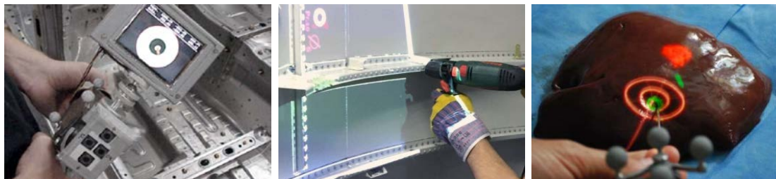
Figure 2.26 – Example of AR industrial applications for maintenance and task assistance: the Intelligent Welding Gun [Echtler et al., 2004] (left), Diota’s projection-based AR assistance for assembly operations (middle) and projection-based AR for medical assistance on liver surgery [Gavaghan et al., 2011] (right).
