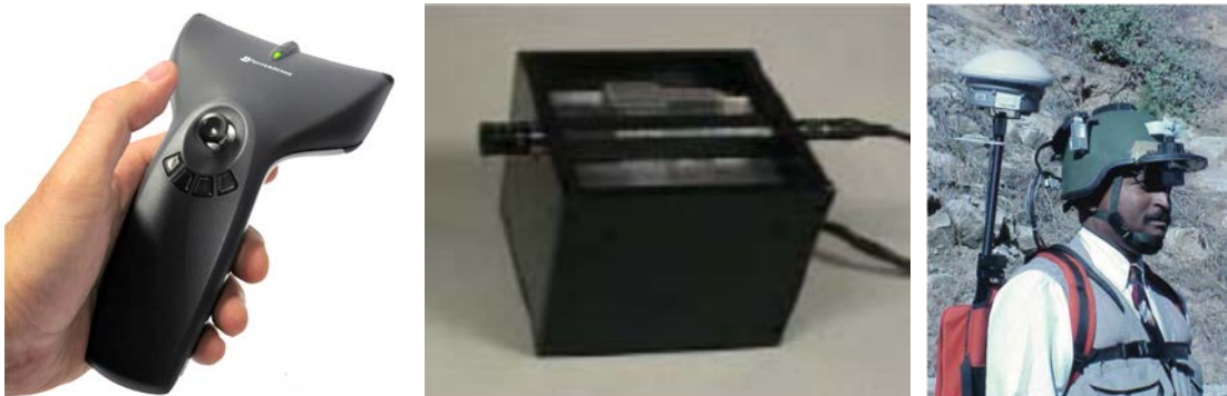
Figure 2.16 – Examples of hybrid tracking devices: the IS-900 acoustic and inertial tracking system from Intersense (left), an inertial and optical tracking system from Jiang et al. [2004] (middle) and the HRL Laboratories tracking device with GPS, inertial and magnetic sensors (right).
